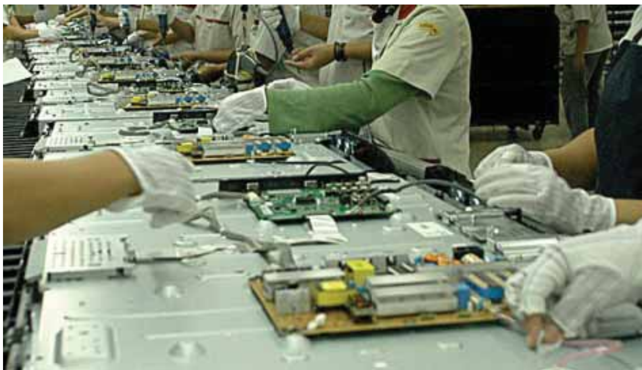
Workers installing the electronic components on the LCD screen in the PT. LG Electronics Indonesia, Cibitung, West Java-Indonesia
